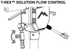
Turn the knob **counter-clockwise** for more flow to clean hightraffic areas. Turn **clockwise** for less flow to clean lower traffic areas.
