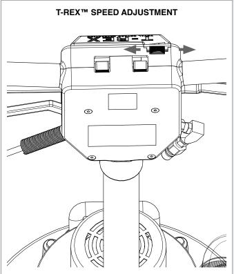
Located at the top of the unit is a speed adjuster. Unit adjusts from 80 - 160 RPM. Move to the left for a slower speed. Move to the right to speed up. Position to desired speed.
