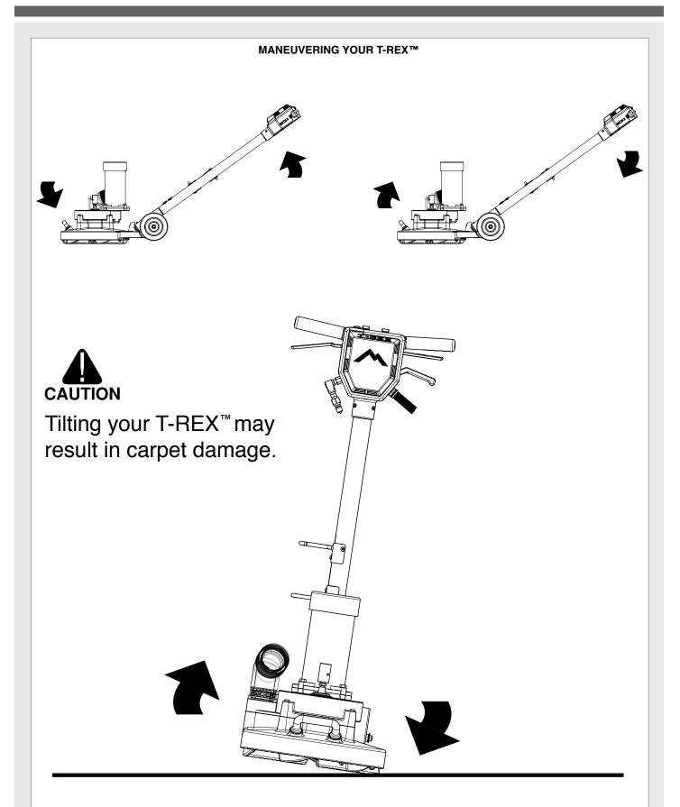
Your T-REX<sup>™</sup> maneuvers much like a floor machine. Slightly lift handle to move to the right. Press the handle down slightly to move to the left. Tilting your T-REX<sup>™</sup> may result in carpet damage. Remember to always keep T-REX<sup>™</sup> evenly balanced on the surface.
