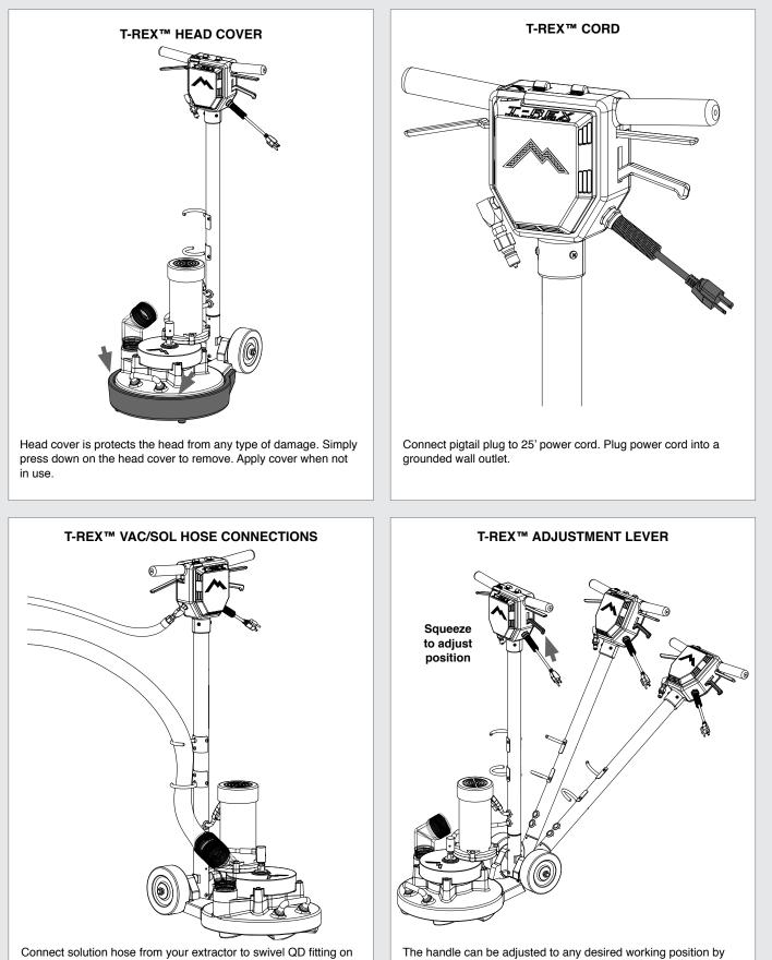
T-REX<sup>™</sup> handle. Also, connect vacuum hose from extractor to Clear View Cuff-Lynx<sup>™</sup> elbow or A105 lead hose.
