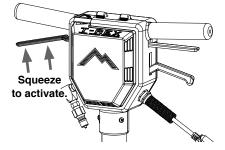
Squeeze lever for solution flow. PSI will be controlled by your extraction unit.
