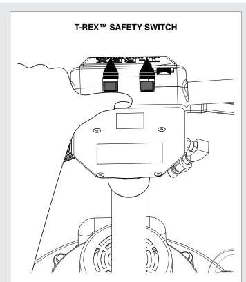
The handle must be lowered to the operating position before switching the machine ON. Disengage the safety switch lock by pushing it forward with either thumb.
