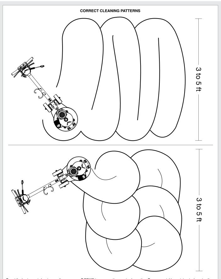
To get the best carpet cleaning results, move your T-REX<sup>™</sup> in an arc pattern or circular motion. To remove stubborn stains, try hovering the T-REX<sup>™</sup> over the stain.
